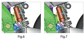
When riding at a fixed speed, the hydraulic cylinder rods are stored to enable smooth riding and counteract any influence on the vehicle's lean. On the other hand, it was confirmed that when vehicle speed is nearly zero, the movements of the swingarms can be controlled by pushing the hydraulic cylinder rods against them, enabling the LMW vehicle to remain upright on its own based on roll rate feedback control (Photo 9).
